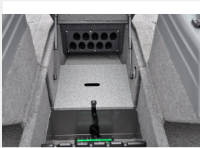
(5) 7'0", (5) 6'0" Lockable in-deck rod locker
